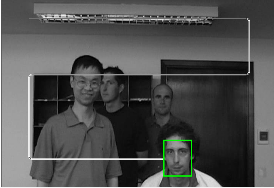
Fig. 7.2 In TLD, a binary ensemble classifier is used to locate the object of interest by applying it in a sliding-window manner. The ability for multi-scale detection is achieved by scaling the size of the detection window. Image is from [282].
